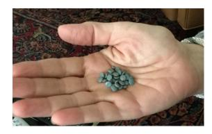
Plastic pellets (aka "nurdles") are produced in the cracker plant.
